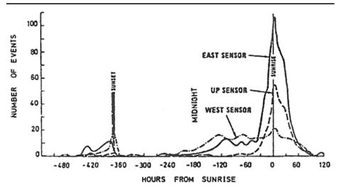
**Fig. 4** Number of particle impacts (events) on the LEAM instrument sensors. Hypervelocity impacts from micrometeorites were rare, but impacts of particles with velocities of up to 1 km/s were detected. After Berg et al. (1976)
