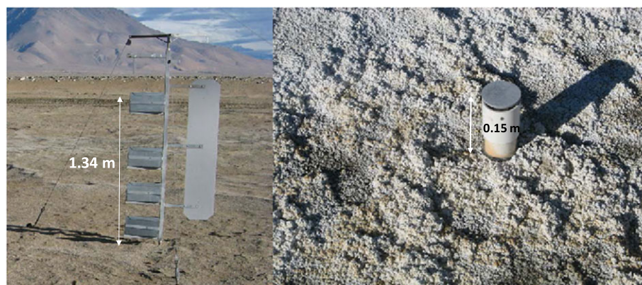
Figure 3. The modified BSNE style trap (left panel) and the Cox Sand Catcher (right panel) used to collect saltating particles. [Colour figure can be viewed at wileyonlinelibrary.com ]
